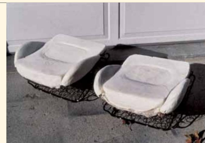
McKeel did not want the look of modern sport seats, so Darin modified the original seats with steel bolsters covered in foam to help keep the driver and passenger in place during spirited rally driving.
