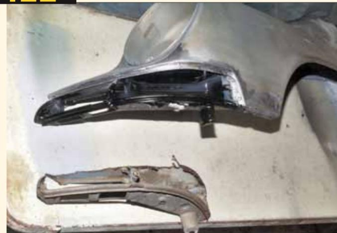
The driver's side front fender was sound, except for the turn signal box. The original pinch welds were recreated by drilling the new part, and plug welding with a MIG welder, Custom's Darin Irvine explains.
