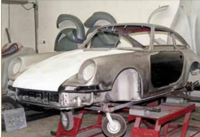
Countless hours were spent adjusting the body before it was ready for the application of primer. The front lid was the original, while the right front fender and front bulkhead were replacement panels.
