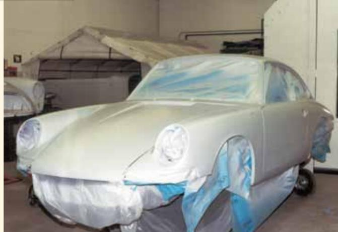
Two coats of PPG DP50 epoxy primer were applied to the entire tub. Then, the exterior panels were sprayed with two to three coats of PPG K36 primer-surfacer, and the body was assembled for final block-sanding.
