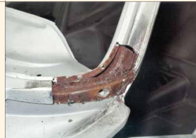
Sandblasting could not touch parts of the inner structure, such as the base of the A pillar. The bodies of 911s have sandwiches of steel in places, which gives them great strength, but makes them tricky to repair.
