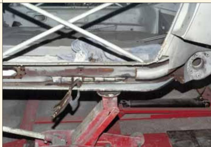
The driver's side heater tube has been removed in preparation for the installation of a new middle sill panel. The floor pans, the same ones installed at the factory, were still sound, and just needed touching up.
