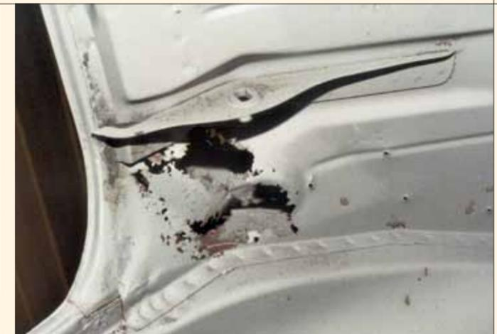
Rust-through in the panel next to the engine lid hinge was exposed by sandblasting. This is a view of the underside of the rear parcel shelf, seen from the engine compartment.
