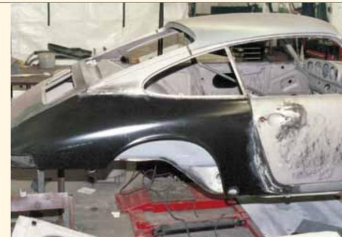
The original rear fenders were damaged beyond economical repair, so a factory replacement pair was installed. After they were welded into place, the seams were filled with lead, as the factory had done.
