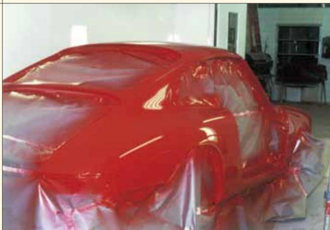
Because Polo Red is nonmetallic, the panels could be painted off the car, allowing no masking lines between the body and jambs. Two coats of PPG DBC basecoat were followed by three coats of PPG 8150 clearcoat.
