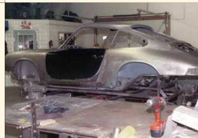
Once the driver's door was re-skinned, the edges were carefully ground and filed to ensure an absolutely perfect door gap. Typically, body panels are assembled and disassembled many times during a restoration.
