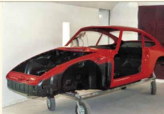
After the clear had cured, it was wet sanded with 1,500-grade paper, using flexible blocks. 3M Perfect-It II polish was applied with a wool finishing pad; a 3M glaze, applied with a waffle pad, was the final touch.
