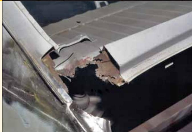
To repair the parcel shelf area, a piece of the outer body at the lower corner of the rear window had to be cut away. The restoration shop fabricated repair panels, and TIG welded them with a Lincoln welder.
