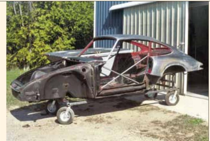
During the second restoration, Custom Automotive Restoration removed the paint with aircraft stripper, cut out rusted sections and braced the door openings before sending the shell out to be media blasted.
