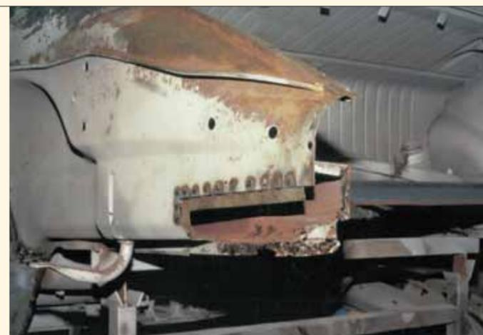
A rusted section of the inner rear fender was cut away and replaced. This area must be absolutely sound, because it supports the rear crossmember, which is crucial to the strength of the back end of the car.
