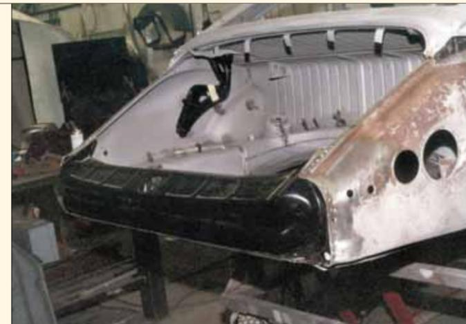
A new, factory crossmember was welded into place. This component carries not only the striker plate mount, but the rear engine mounts. "It's a structurally important part of the car," Darin explains.
