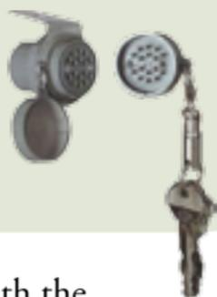
channeled through the master unit. With the plug removed, the circuits are broken, preventing current from flowing. As additional protection, because all wires in the Ravelco harness are the same color and within a steel-encased harness, it is incredibly difficult to jump the wires and complete the circuits needed to start the car. For additional information on the Ravelco Anti-Theft Device, visit [www.ravelco.com](http://www.ravelco.com).
