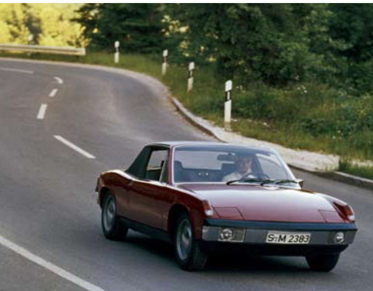
The 1970–76 914 (top) was Porsche's first true production mid-engined car, with a horizontally opposed engine, two trunks and a clever removable top.
