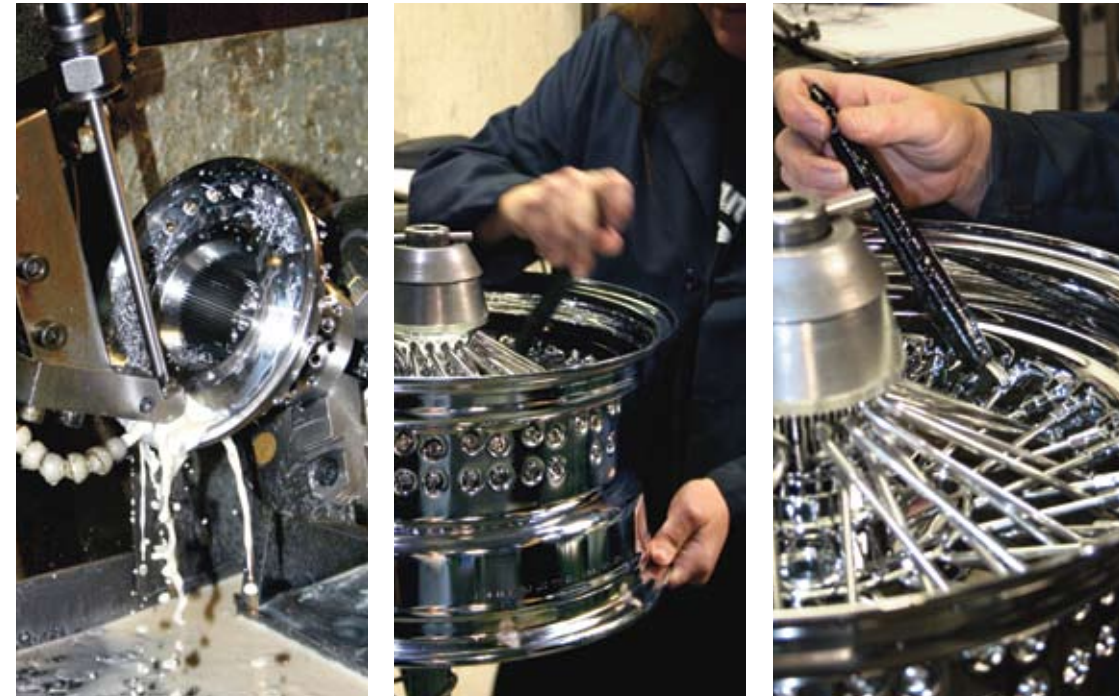
Part of building a new wire wheel includes (from left) drilling a hub to accept the spokes, tightening the spokes and then adjusting them until the wheel is true.
