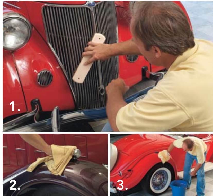
Pictures 1 & 2: Wash your car with a Boar's hair brush, soft sponges or sheepskin mitts to protect its finish. Picture 3: Be sure to dry the surface with a chamois — it's much easier to use than an absorbent towel.
