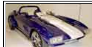
1963 Corvette Grand Sport Replica , tube frame, LT-1 engine, 6 speed tranny, ZR-1 suspension. Dana rear, XM digital satellite multimedia system. Custom forged aluminum wheels. Integrated roll bar.
